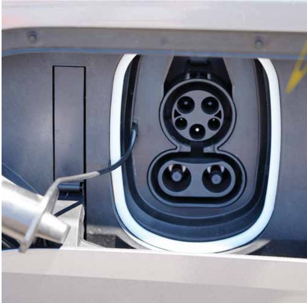
▲ Charging receptacle in car with Levels 1, 2 and 3 options available. On this vehicle, the top round receptacle is used for Level 1 and 2 charging. Both receptacles are used for the fastest, Level 3 charging.
